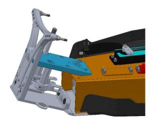
Steering levers are put on the master and slave axle with the bearings. The top deck is placed over the axles and mounted to the front bulkhead and top deck.
