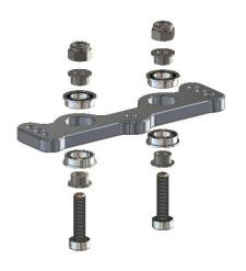
The steering plate is prepared as shown on the left.
