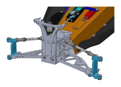
Press in bushings into the c-hub and mount the c-hub between upper and lower wishbone.
