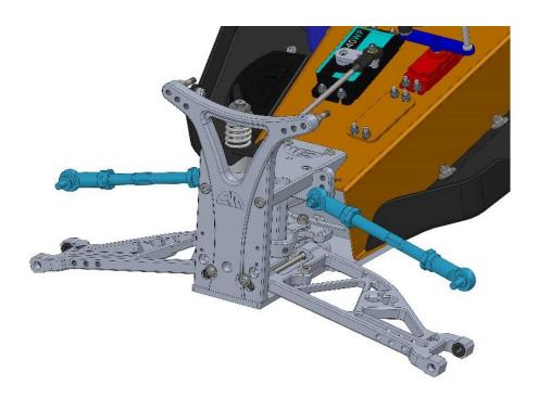
Assemble the upper wishbone linkages with the M8 L/R nuts and the L/R ball joints.
