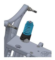
Fix the alloy bottom part of the servo saver to the main shaft. Place the plastic top part onto it.
