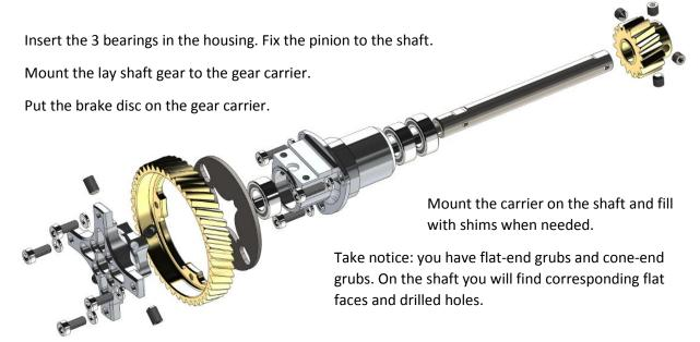
Mount the pre-assembled lay shaft into the main gear plate.
